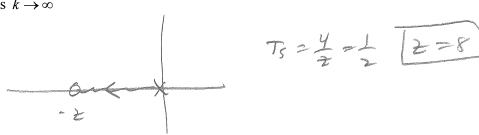
b) Assuming a the PI controller  $G_c(s) = \frac{k(s+z)}{s}$ , what is the value of z so that the settling time  $T_s = 0.25$  as  $k \to \infty$
