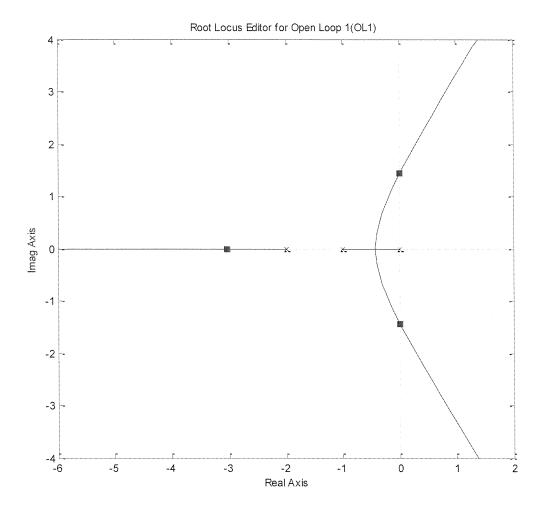
7) Is it possible for -3 to be a closed loop pole for this system? (Yes or No)
