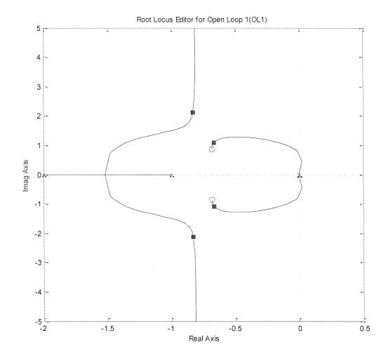
10) When k = 3.5 the poles are as they are shown in the figure. Estimate the closed loop poles.
