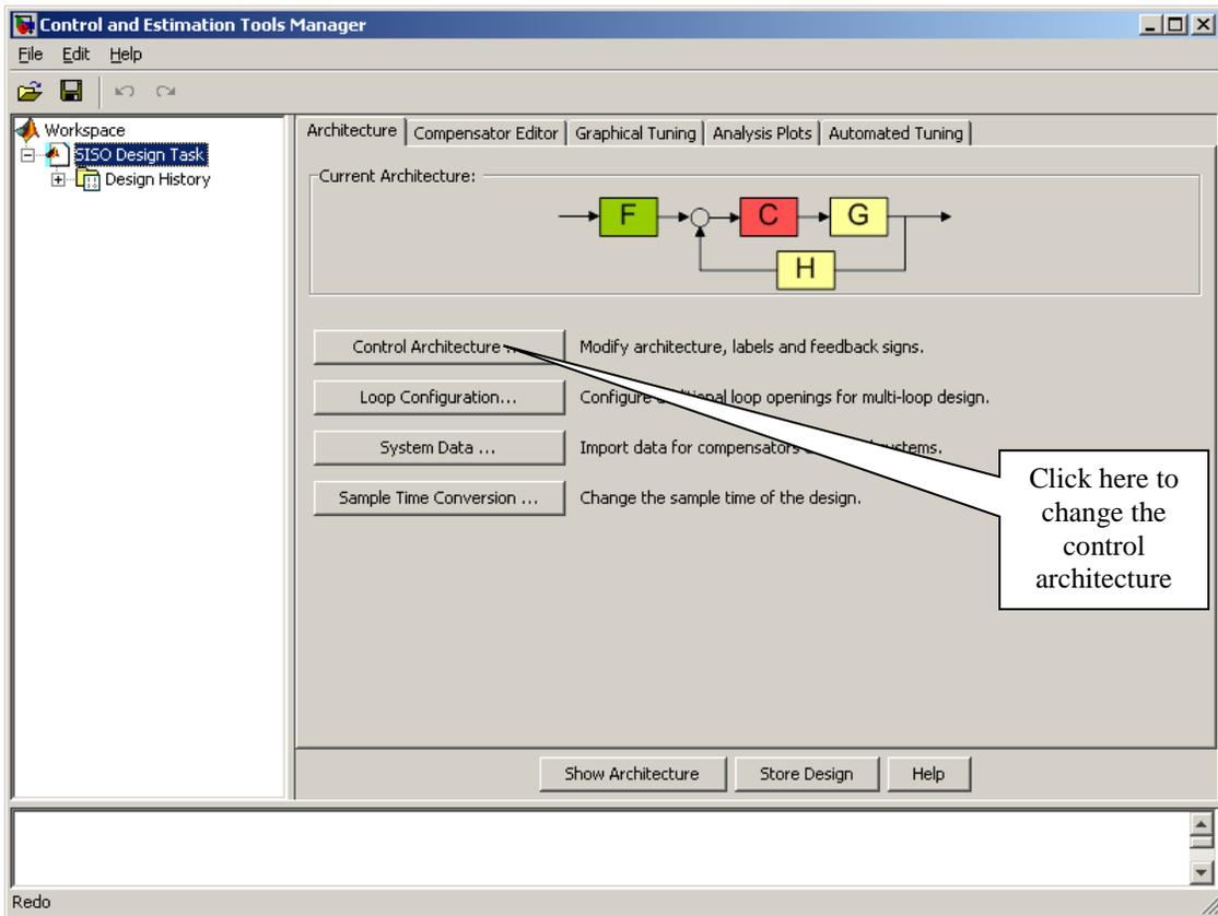
Next we need to select the correct architecture. Select the following architecture and be sure that *sisotool* uses negative feedback for both loops.
