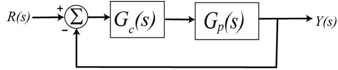
a) Determine the closed loop transfer function,  $G_0(s)$
