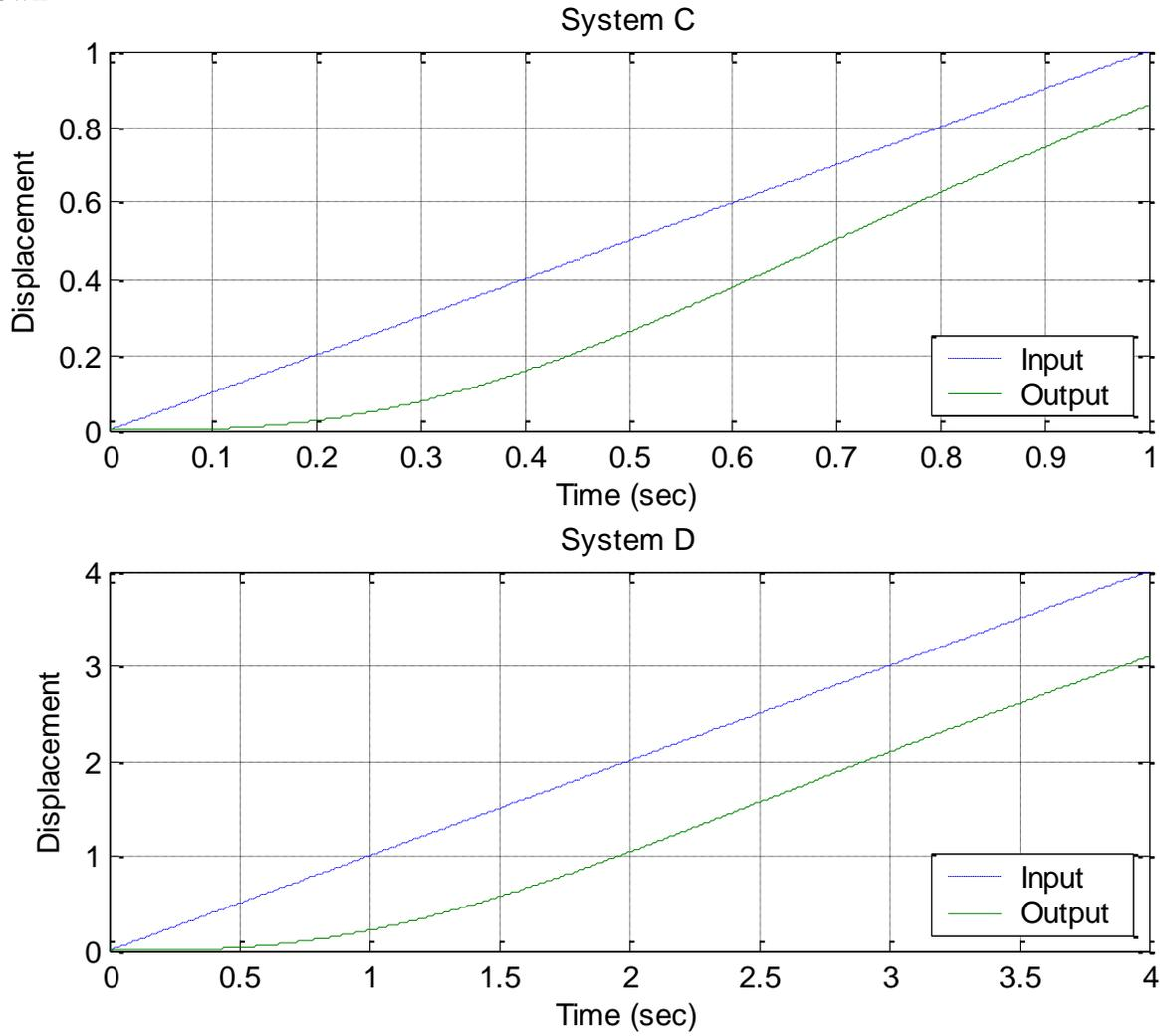
**Figure 2.** Ramp responses for systems C and D.
