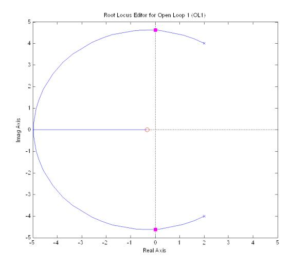
5) Assume we are adding a lag compensator to change the steady state error for a ramp input, as shown below
