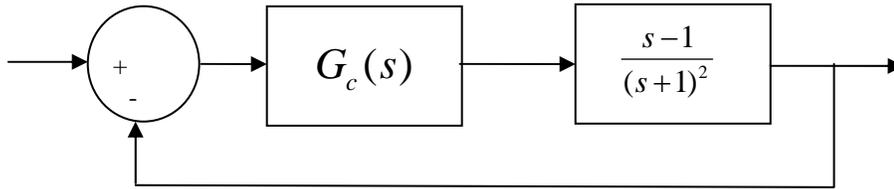
1) If we want the minimum order controller to place the closed loop poles (and have a type 0 system), the controller will have which of the following forms
