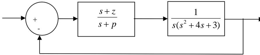
Assume we want to use the lag compensator so that the steady state error for a unit ramp is  $e_{ss} = 0.1$ . We will be varying the locations of the pole and zero of the lag compensator to accomplish this, and will look at the effects of these changes on both the unit step response and the unit ramp response. For each of the simulations below, run the simulation to 35 seconds. For  $z = 0.1, 0.01, \text{ and } 0.001$
