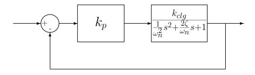
a) Show that the sensitivity of the closed loop system to  $k_{clg}$  is
