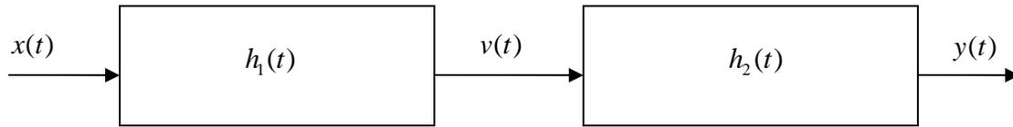
Determine the impulse response  $h(t)$  of the entire system if the impulse responses of the subsystems are given as:
