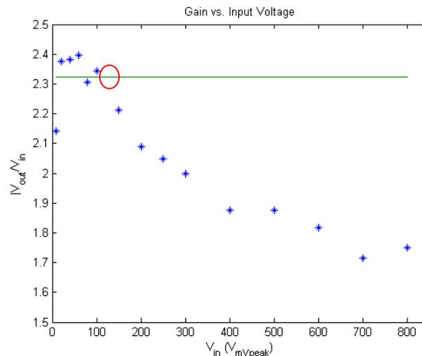
d) You can get a rough estimate of the gain compression point by looking at your plot. This point is defined as the input voltage at which the gain begins to decrease and is indicated by the red circle in the figure above. You should indicate your gain compression point similarly in your plot. Use the menu commands in the figure window to insert an ellipse.
