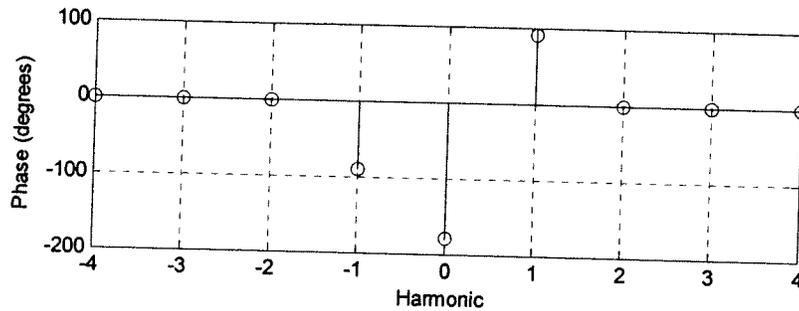
The system transfer function,  $H(k\omega_0)$ , has the following spectrum:
