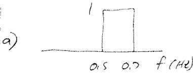
Remove all signals with frequencies outside 0.5 to 0.7 Hz
