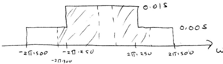
$$\begin{aligned} E_{\text{total}} &= \frac{1}{2\pi} \int_{-2\pi/500}^{2\pi/500} |\bar{X}(w)|^2 dw = \frac{1}{2\pi} \left[ 2 \cdot \int_{-2\pi/300}^{-2\pi/250} (0.005)^2 dw + 2 \int_{2\pi/250}^{2\pi/500} (0.015)^2 dw \right] \\ &= \frac{1}{2\pi} \left[ 2 \cdot (2\pi/250)(0.005)^2 + 2 \cdot (2\pi/250)(0.015)^2 \right] \\ &= 2 \cdot 250 \cdot (0.005)^2 + 2 \cdot 250 \cdot (0.015)^2 = \boxed{0.125 = E_{\text{total}}} \end{aligned}$$
