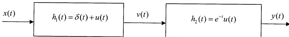
Determine the impulse response of the **system** ( relating  $y(t)$  and  $x(t)$  ).
