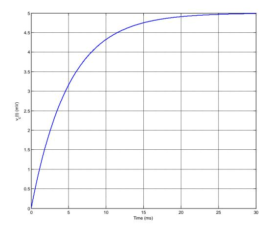
Based on this figure, the best estimate of the **time constant** for this system is
