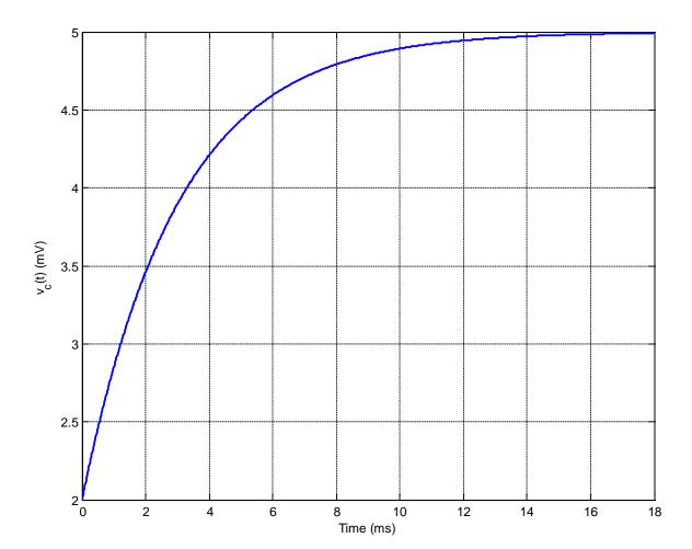
Based on this figure, the best estimate of the **time constant** for this system is
