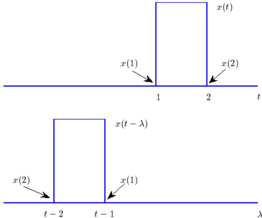
**Figure 5.7.** Input signal for Example 5.5.2. The original signal  $x(t)$  is shown in the top panel, with the two convenient “marker” points. The lower panel shows  $x(t - \lambda)$  as a function of  $\lambda$ , and shows how these marker points move as the parameter  $t$  is varied. Note that the function  $x(t)$  has been flipped (reversed) from its original orientation.
