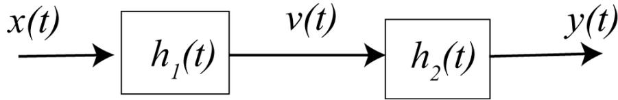
**Figure 5.21.** Two LTI systems connected in series.
