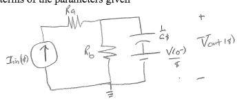
$$Iin 18) = \frac{V_{out18}}{R_b} + \frac{V_{out18} - V_{10}}{8} = \overline{V_{out18}} \left[ \frac{1}{R_b} + C4 \right] - V_{10} C$$
