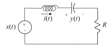
For this circuit, use your **variable resistor** for R, use a 0.01  $\mu$ f capacitor, and a 33 mH inductor. For this system the transfer function is
