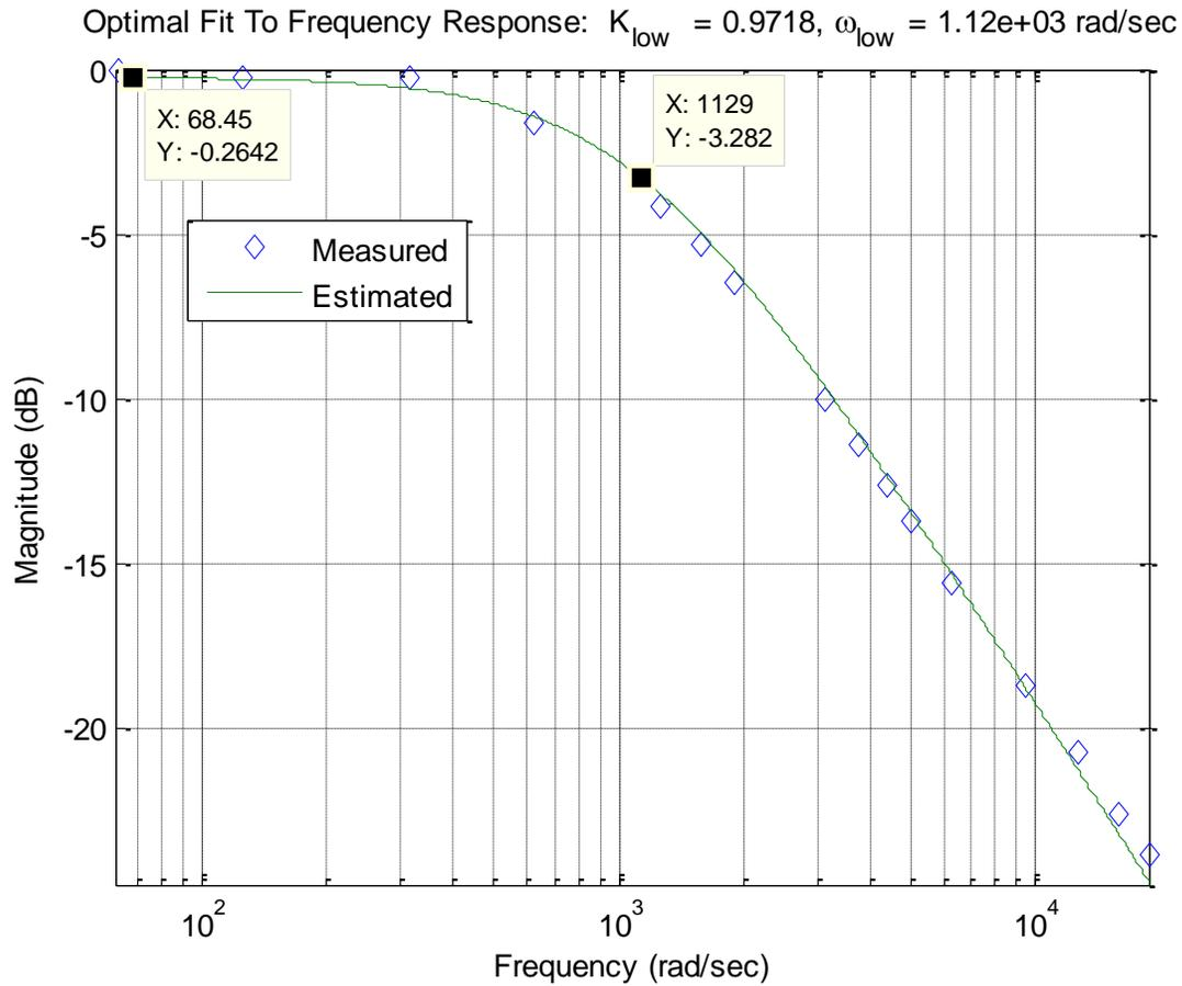
**Figure 3.** The lowpass filter with a bandwidth of approximately 1130 rad/sec (180 Hz).
