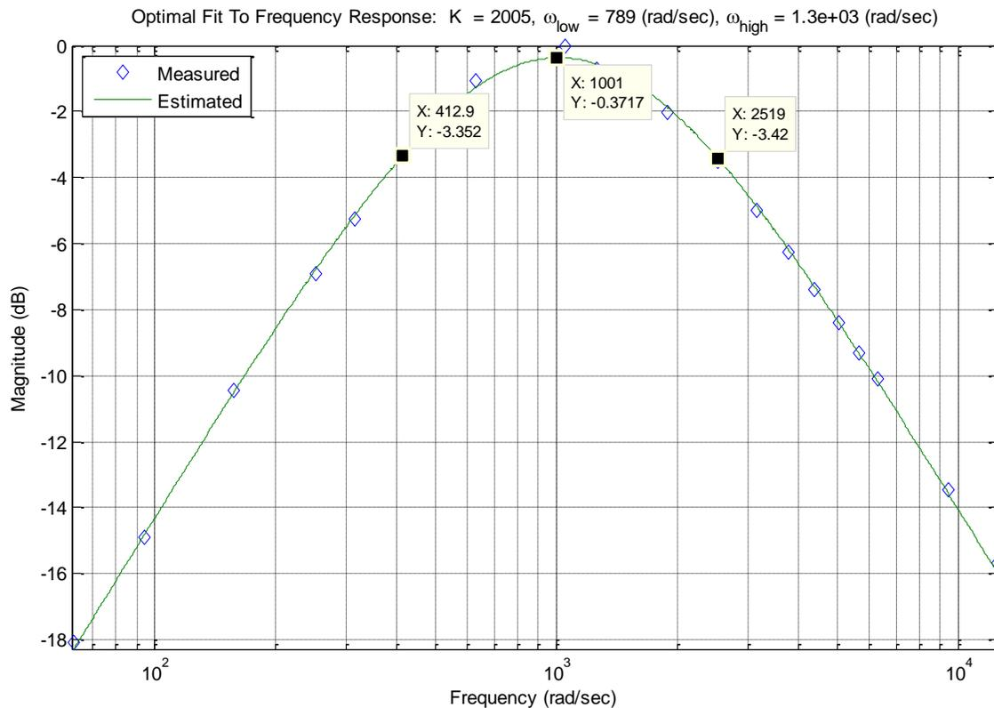
**Figure 8.** Bandpass filter with both low and high cutoff frequencies identified. The bandwidth of this system is approximately 2106 rad/sec (335 Hz). Note that this is not a very good bandpass filter.
