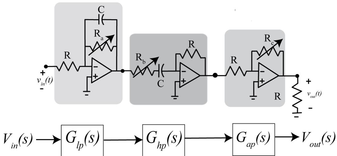
**Figure 1.** Bandpass filter consisting of a lowpass filter, a highpass filter, and an all pass (gain) filter.
