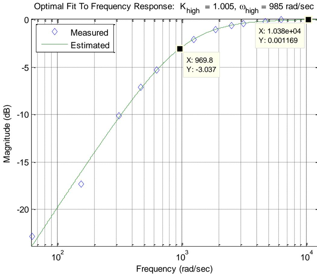
**Figure 5:** Highpass filter with a cutoff frequency of approximately 970 rad/sec (154 Hz).
