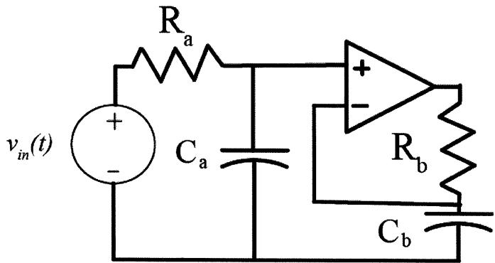
$$V^+ = \frac{\frac{1}{C_a s}}{R_a + \frac{1}{C_a s}} V_{in}(s)$$
