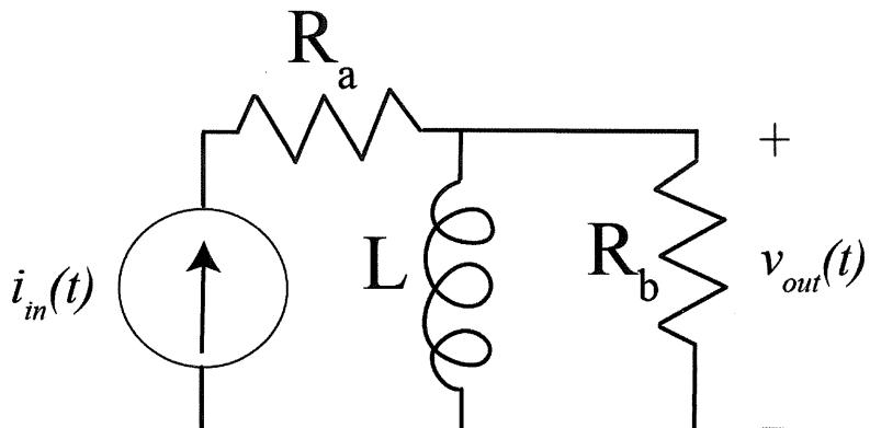
$$\frac{V_{out}(s)}{R_b} + \frac{V_{out}(s)}{Ls} = I_{in}(s)$$
