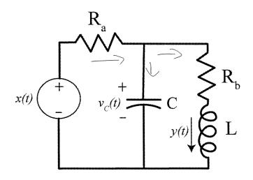
$$\frac{x - k}{Ra} = C \frac{\partial c}{\partial t} + y \qquad V_c - yk_b - k\dot{y} = 0$$
