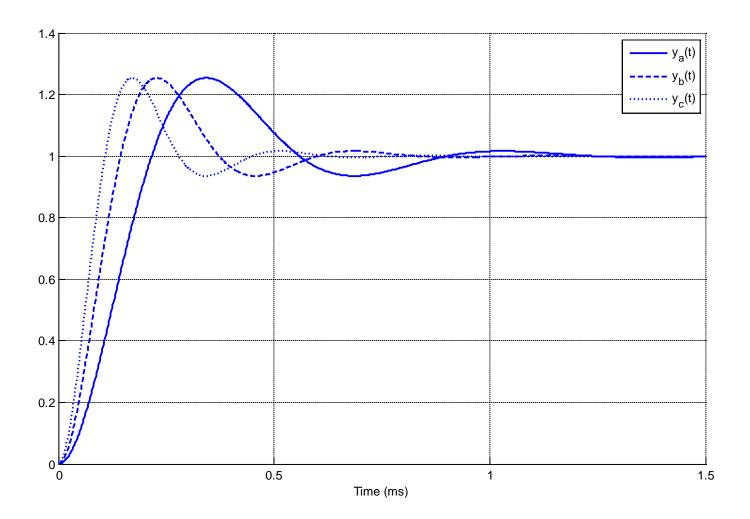
Problems 13 and 14 refer the following graph showing the response of a second order system to a step input.
