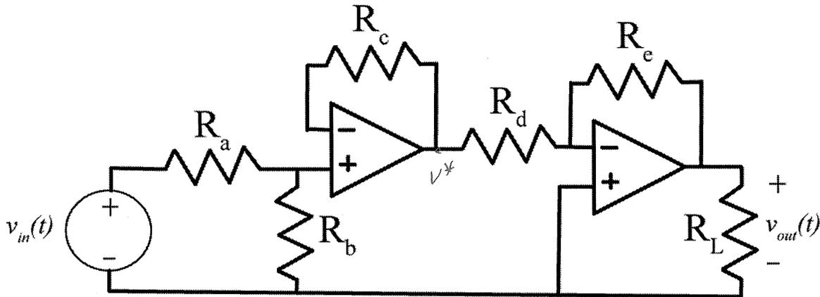
$$V^* = \frac{V_{in} R_b}{R_a + R_b} \quad \frac{V^*}{R_d} + \frac{V_{out}}{R_e} = 0 \quad V_{out} = -\frac{R_e}{R_d} V^* = \left[ -\frac{R_e}{R_d} \frac{R_b}{R_a + R_b} \right] V_{in}$$
