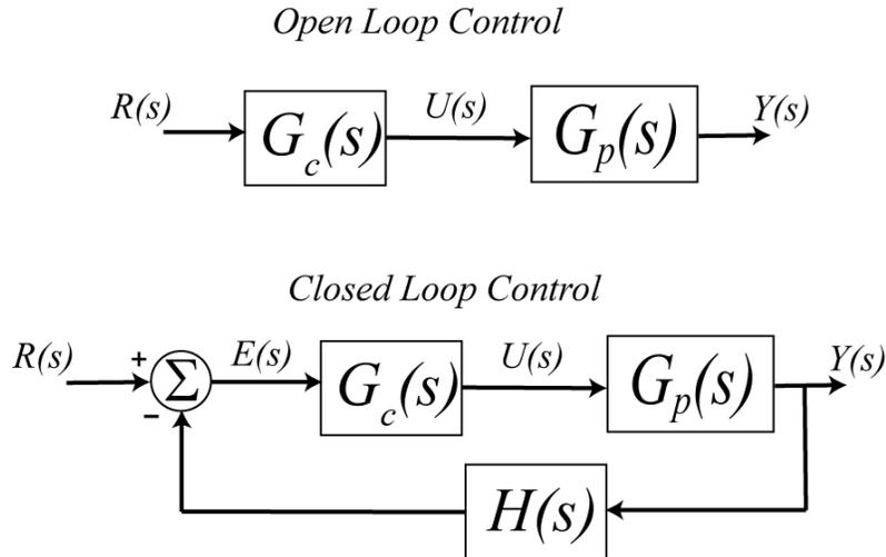
**Figure 7.23.** Open loop and closed loop control of a plant. Here  $r(t)$  is the reference input,  $u(t)$  is the control effort or control signal,  $y(t)$  is the system output, and  $e(t)$  is the error signal. Often the transfer function in the feedback loop,  $H(s)$ , is some type of transducer which converts the output to the same form at the input.
