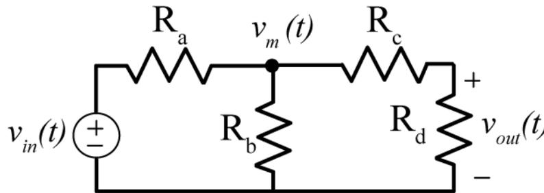
**Figure 7.20.** Circuit used to demonstrate loading.
