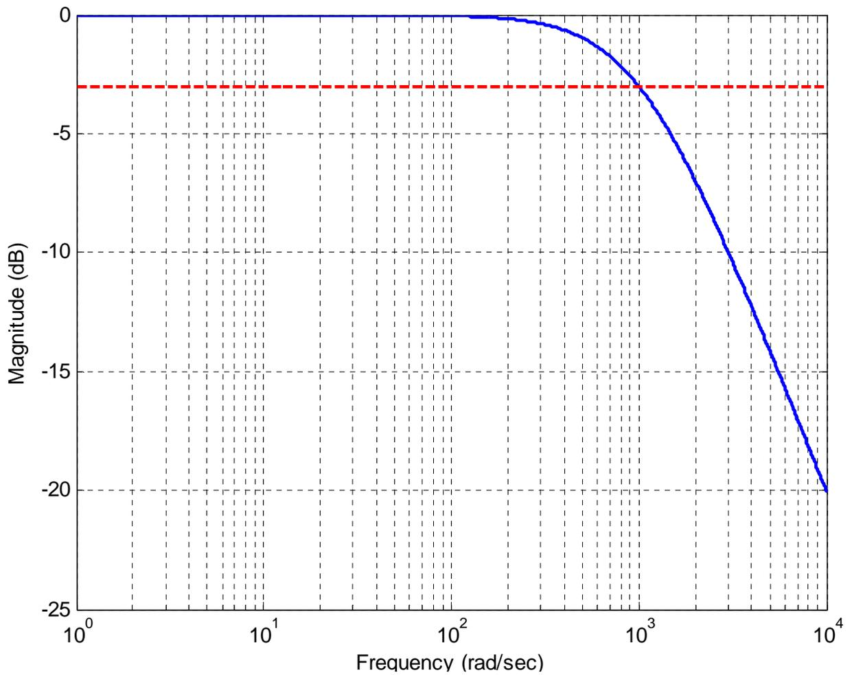
**Figure 8.21.** Bode plot of the magnitude of the transfer function for Example 8.6.1. The maximum value of the transfer function is 1 (0 dB), so the bandwidth will be determined by the point where the magnitude falls to  $-3$  dB. This occurs at 1000 rad/sec.
