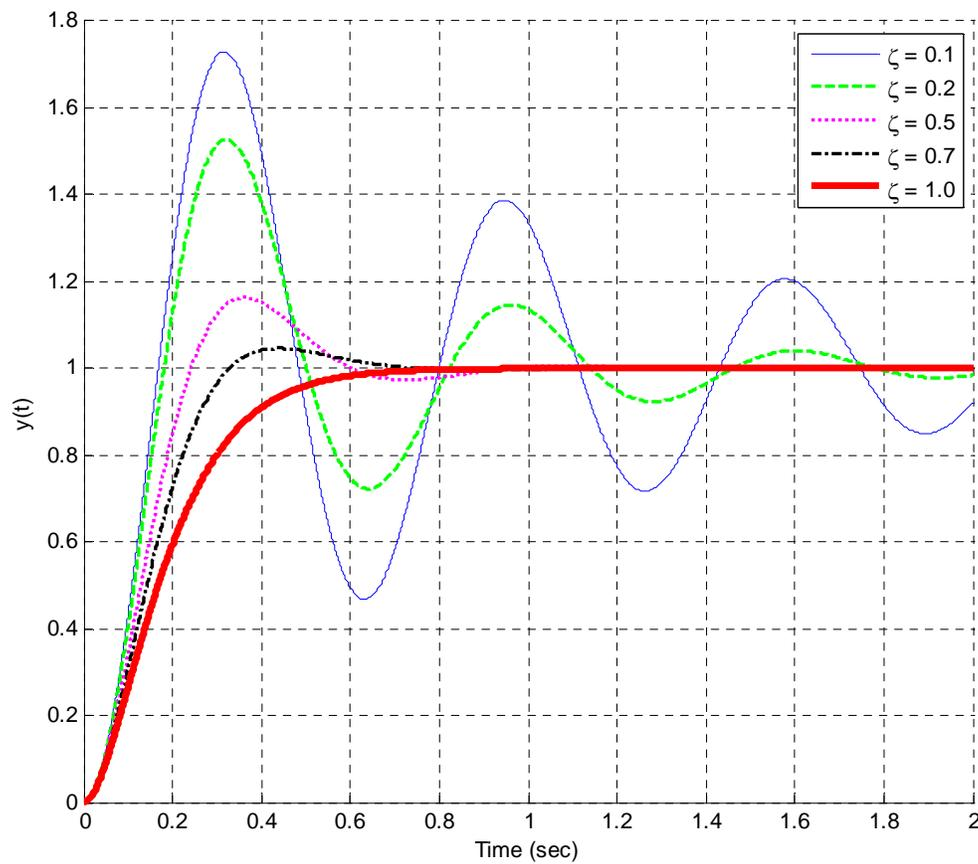
**Figure 3.6.** The response (output) of a system initially at rest. For this system  $KA = 1$  and  $\omega_n = 10$  rad/sec. There are four responses for under damped systems ( $0 < \zeta < 1.0$ ) and one response for a critically damped system ( $\zeta = 1.0$ ). The only thing changing in the responses is the damping ratio.
