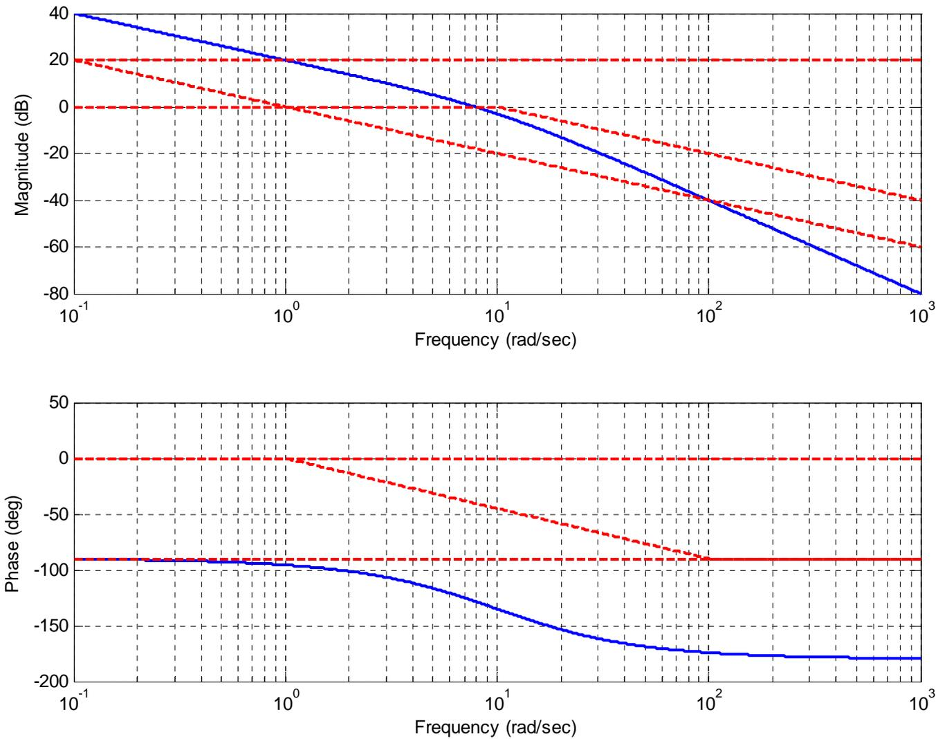
**Figure 8.15.** Bode plot for the transfer function  $G(s) = \frac{100}{s(s+10)} = \frac{10}{s(0.1s+1)}$ . The straight line approximations of the individual components are shown as dashed lines, the actual Bode plot is shown as a continuous line. Note that for any given frequency, if you sum the values of the straight line approximations you get reasonable approximations to the true (continuous curve) Bode plot.
