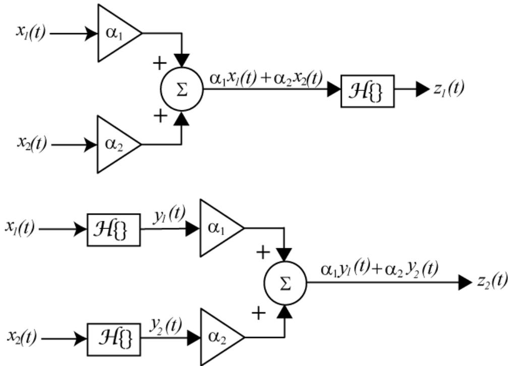
**Figure 4.5.** Signal flow graph of linearity test.
