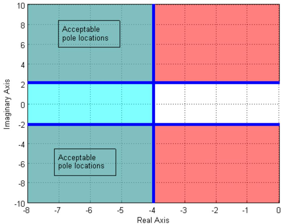
**Figure 7.12.** The pole locations corresponding to a maximum time to peak of 1.5 seconds and a settling time less than 1 seconds. The settling time constraint means the real part of the poles must be less than -4, and the peak time constraint means the absolute value of the imaginary part of the pole must be greater than 2.09. The pole locations that meet both of these constraints is the overlapping regions, labeled as “Acceptable pole locations”.
