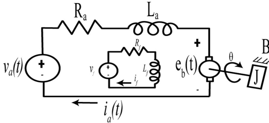
**Figure 7.18.** Model of an armature controlled DC motor.
