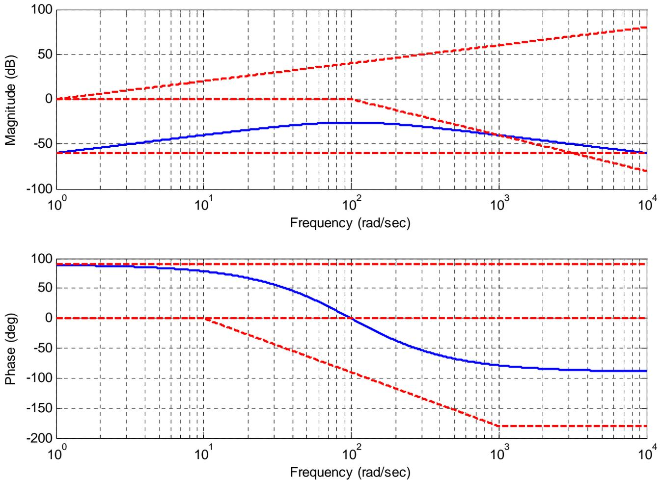
**Figure 8.17.** Bode plot for the transfer function.  $G(s) = \frac{10^{-3}s}{(0.01s+1)^2}$  The straight line approximations of the individual components are shown as dashed lines, the actual Bode plot is shown as a continuous line. Note that for any given frequency, if you sum the values of the straight line approximations you get reasonable approximations to the true (continuous curve) Bode plot.
