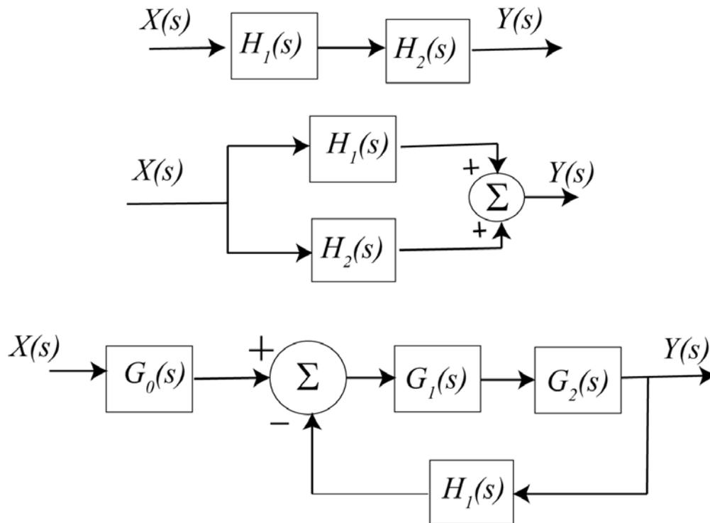
**Figure 6.12.** Transform domain representation of systems from Figure 6.11.
