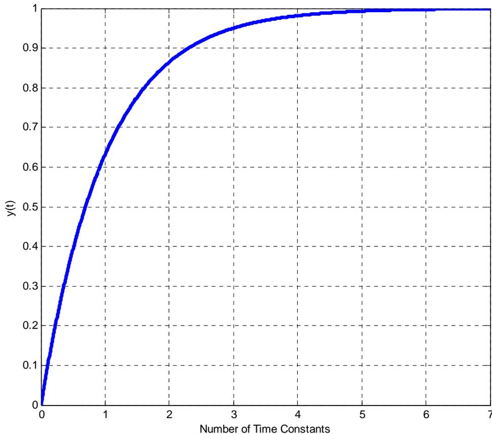
**Figure 2.6.** Graph of  $y(t) = 1 - e^{-t/\tau}$  for  $t = 0\tau$  up to  $t = 7\tau$ .  $y(t)$  is within 5% of its final value in 3 time constant, within 2% of its final value in 4 time constants, and within 1% of its final value in 5 time constants.
