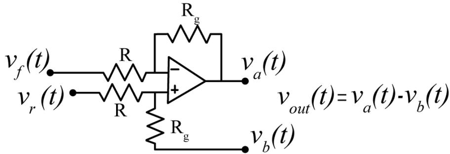
**Figure 7.16.** Differential amplifier circuit used in Example 7.7.3.
