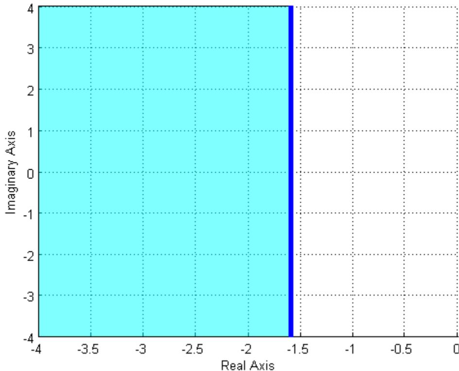
**Figure 7.6.** The pole locations corresponding to a settling time less than 2.5 seconds are shown in the shaded region, to the left of -1.6 on the real axis. Note that the settling time constraint only affects the real part of the pole, not the imaginary part of the poles.
