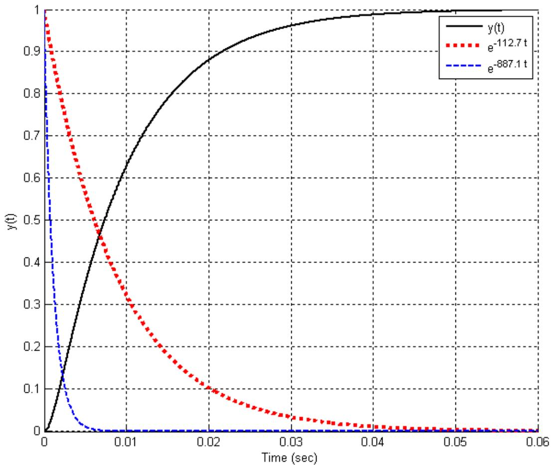
**Figure 3.12.** Response of system analyzed in Example 3.5.4 and plots of the exponentials that make up the response. For this system,  $y(t) = 1 - 1.145e^{-112.7t} + 0.145e^{-887.1t}$ . This system has components with time constants  $\tau = \frac{1}{112.7} = 0.00887 \text{ sec}$  and  $\tau = \frac{1}{887.1} = 0.00113 \text{ sec}$ . The response of the system is clearly dominated by the component of the response with the largest time constant.
