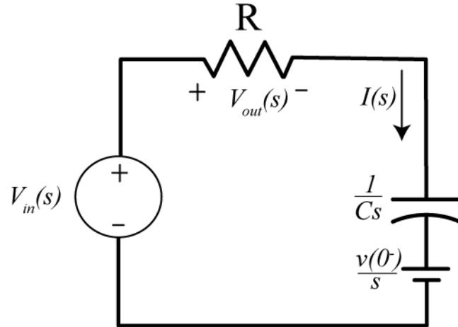
**Figure 6.5.** Circuit from Example 6.3.1 in the Laplace domain.
