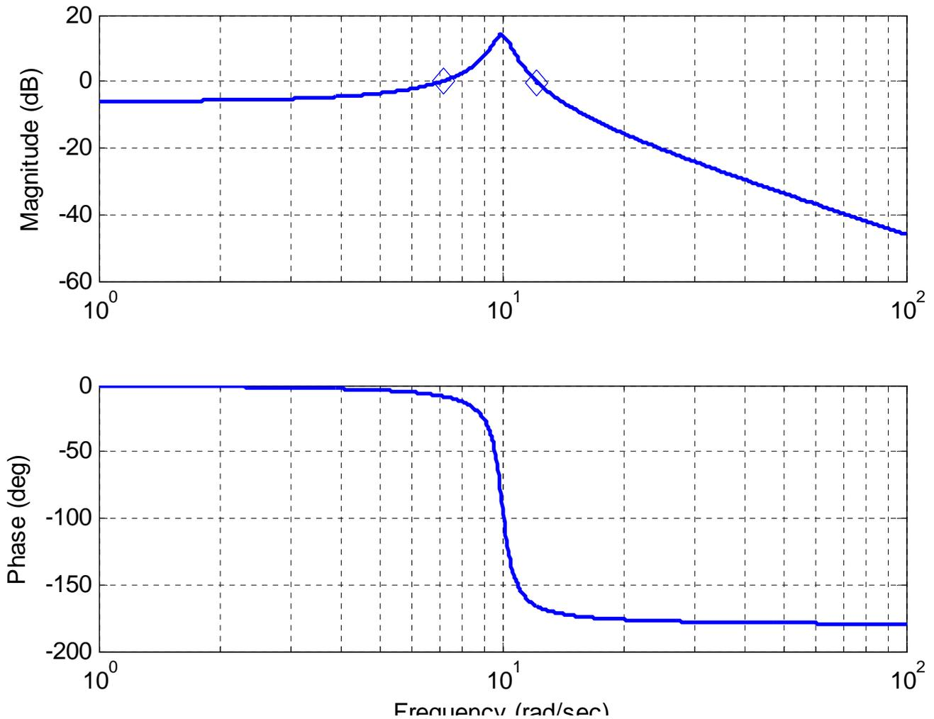
**Figure 8.27.** Bode plot for Example 8.7.2. The gain crossover frequencies are shown as diamonds. There is no phase crossover frequency. The phase margin for this system is approximately 14 degrees, and the gain margin is infinite.
