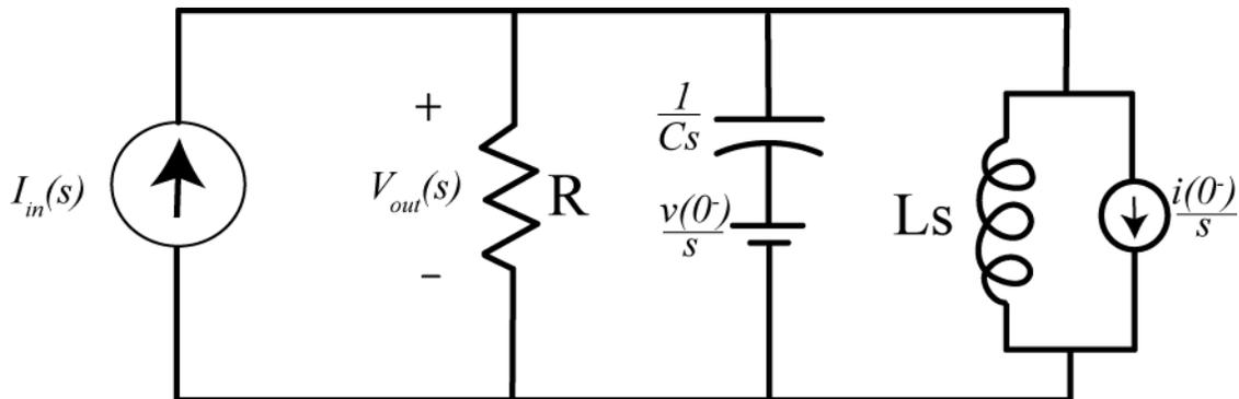
**Figure 6.9.** Circuit from Example 6.3.3 in the Laplace domain.
