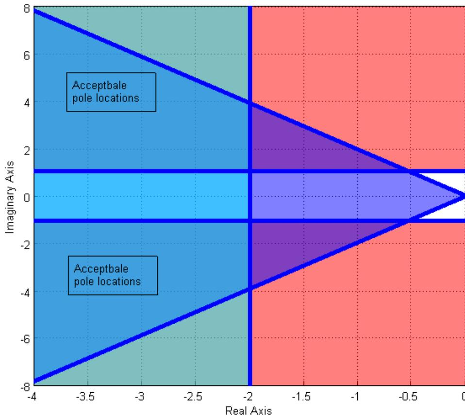
**Figure 7.13.** The acceptable pole locations for an ideal second order system that corresponds to a time to peak of less than or equal to 3 seconds, a settling time of less than 2 seconds, and a percent overshoot of less than 20%. The pole locations that meet all of these constraints is the overlapping regions, labeled as “Acceptable pole locations”.
