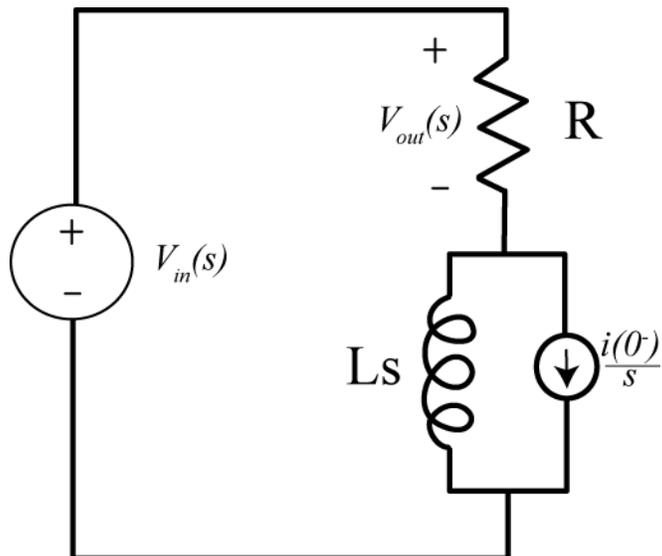
**Figure 6.7.** Circuit from Example 6.3.2 in the Laplace domain.
