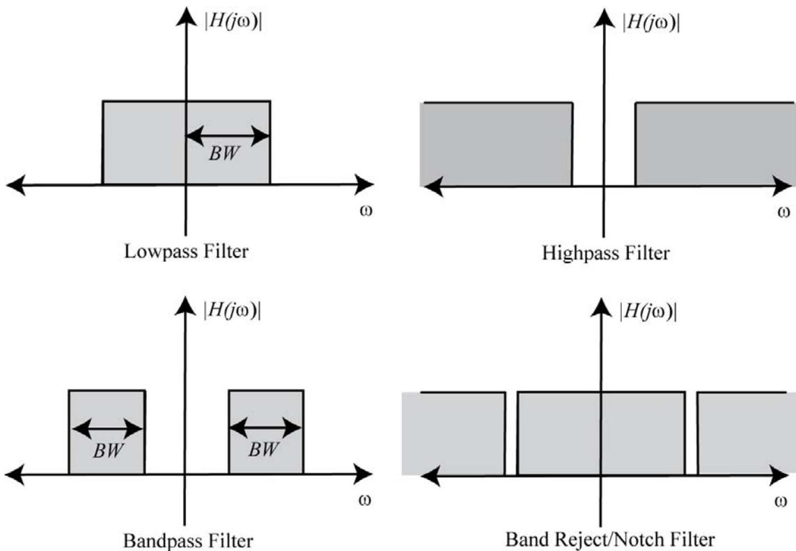
**Figure 8.23.** Ideal lowpass, highpass, bandpass, and bandreject filters.
