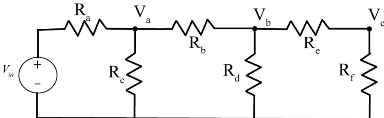
c) Create m-files to set up and solve matrix equations for the node values for the following circuit. Use ***both*** methods from the Appendix to set up the system of equations.
