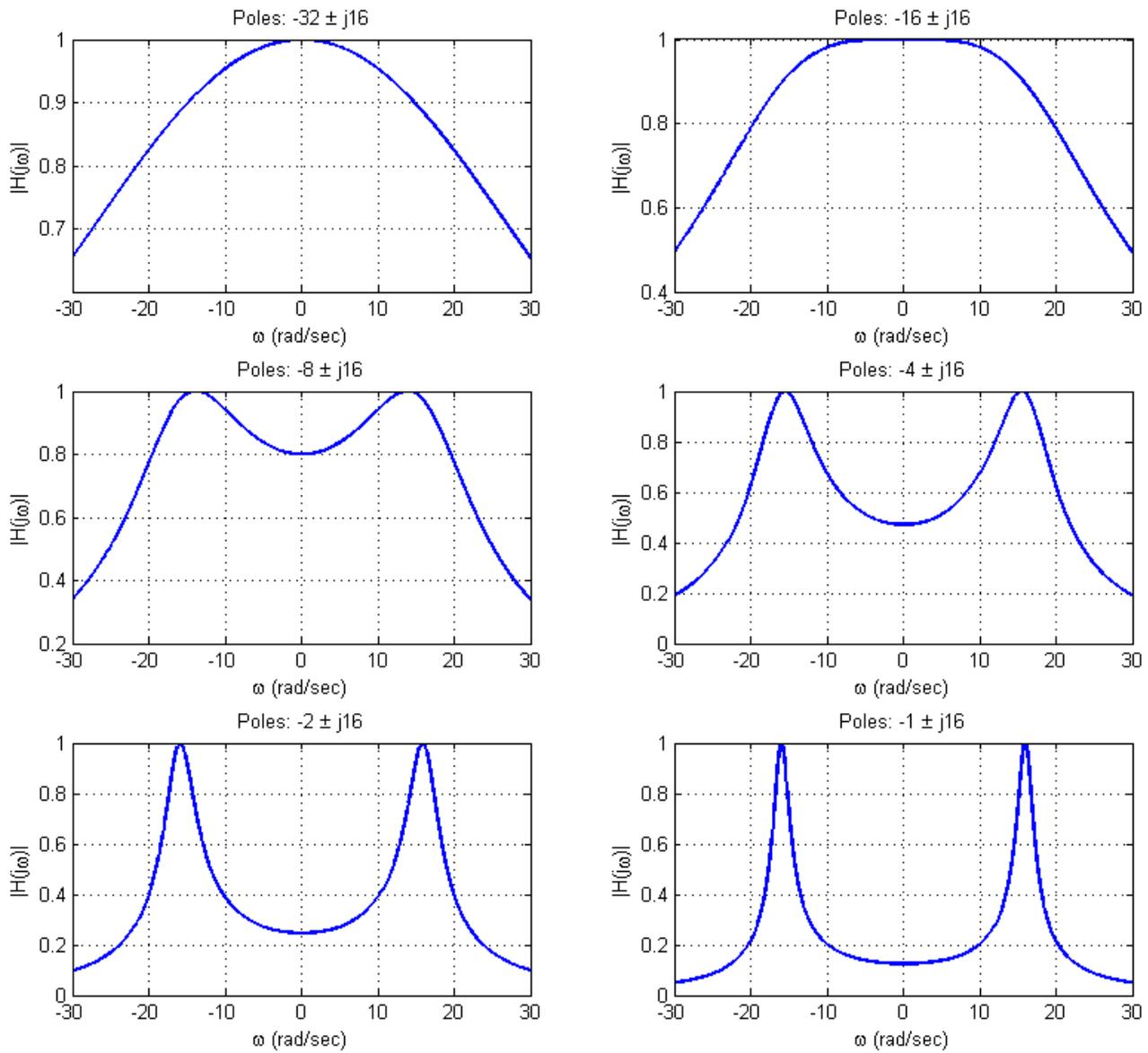
**Figure 8.9.** This figure shows the magnitude of the frequency response of various systems that have two complex conjugate poles. All of these systems have poles of the form  $\sigma \pm j16$  where the real part of the pole varies from  $-32$  to  $-1$ . The magnitudes for these systems have been scaled to have a maximum value of one.
