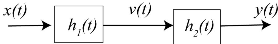
**Figure 5.21.** Two LTI systems connected in series.
