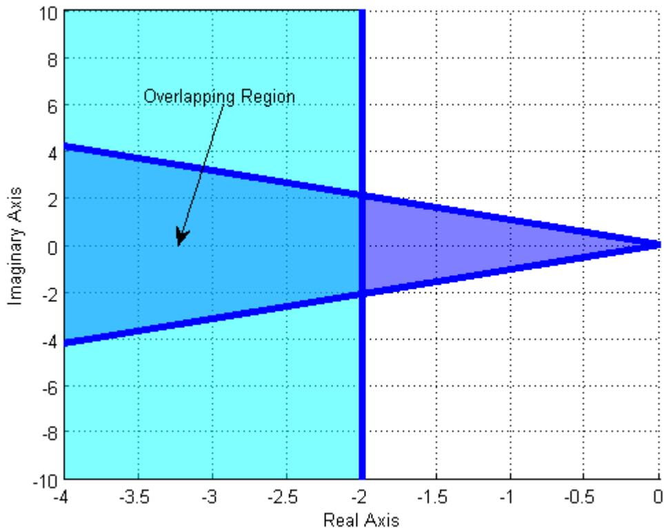
**Figure 7.10.** The pole locations corresponding to a maximum percent overshoot of 5% and a settling time of 2 seconds are shown in the shaded regions. The overlapping region shows the location in the s-plane where both conditions are met.
