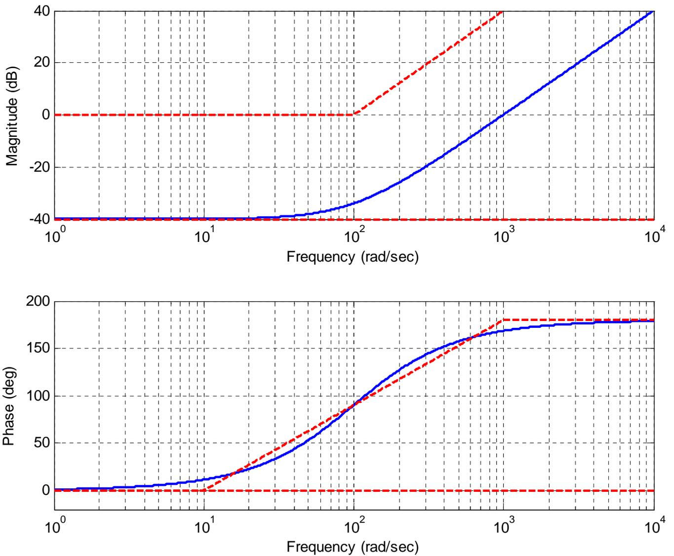
**Figure 8.14.** Bode plot for the transfer function  $G(s) = \frac{1}{100} \left( \frac{1}{100} s + 1 \right)^2$ . Note the 6 dB discrepancy at the corner frequency in the magnitude plot. The straight line approximations of the individual components are shown as dashed lines, the actual Bode plot is shown as a continuous line. Note that for any given frequency, if you sum the values of the straight line approximations you get reasonable approximations to the true (continuous curve) Bode plot.
