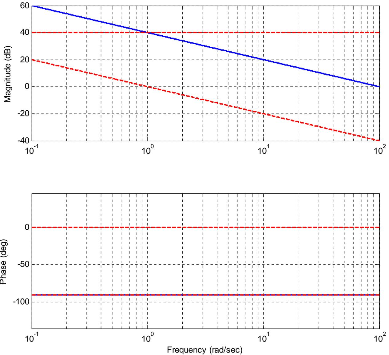
**Figure 8.12.** Bode plot of the transfer function  $G(s) = \frac{100}{s}$ . The Bode plots of the two subcomponents are shown as dashed lines, the final Bode plot is shown as a solid line. In the phase diagram, the subcomponent at -90 degrees overlaps with the final phase of -90 degrees (since the other subcomponent's phase is zero). Note that the sum of any two values (at a given frequency) on the dashed lines equals the value on the solid line at the same frequency.
