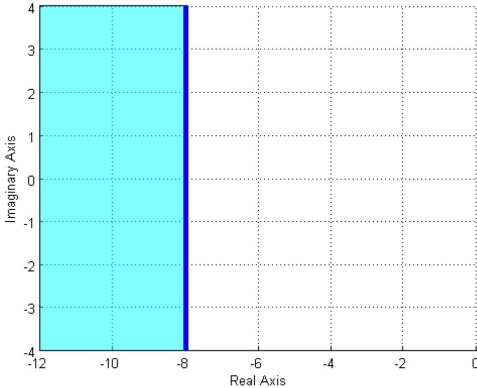
**Figure 7.7.** The pole locations corresponding to a settling time less than 0.5 seconds are shown in the shaded region, to the left of -8 on the real axis. Note that the settling time constraint only affects the real part of the pole, not the imaginary part of the poles.
