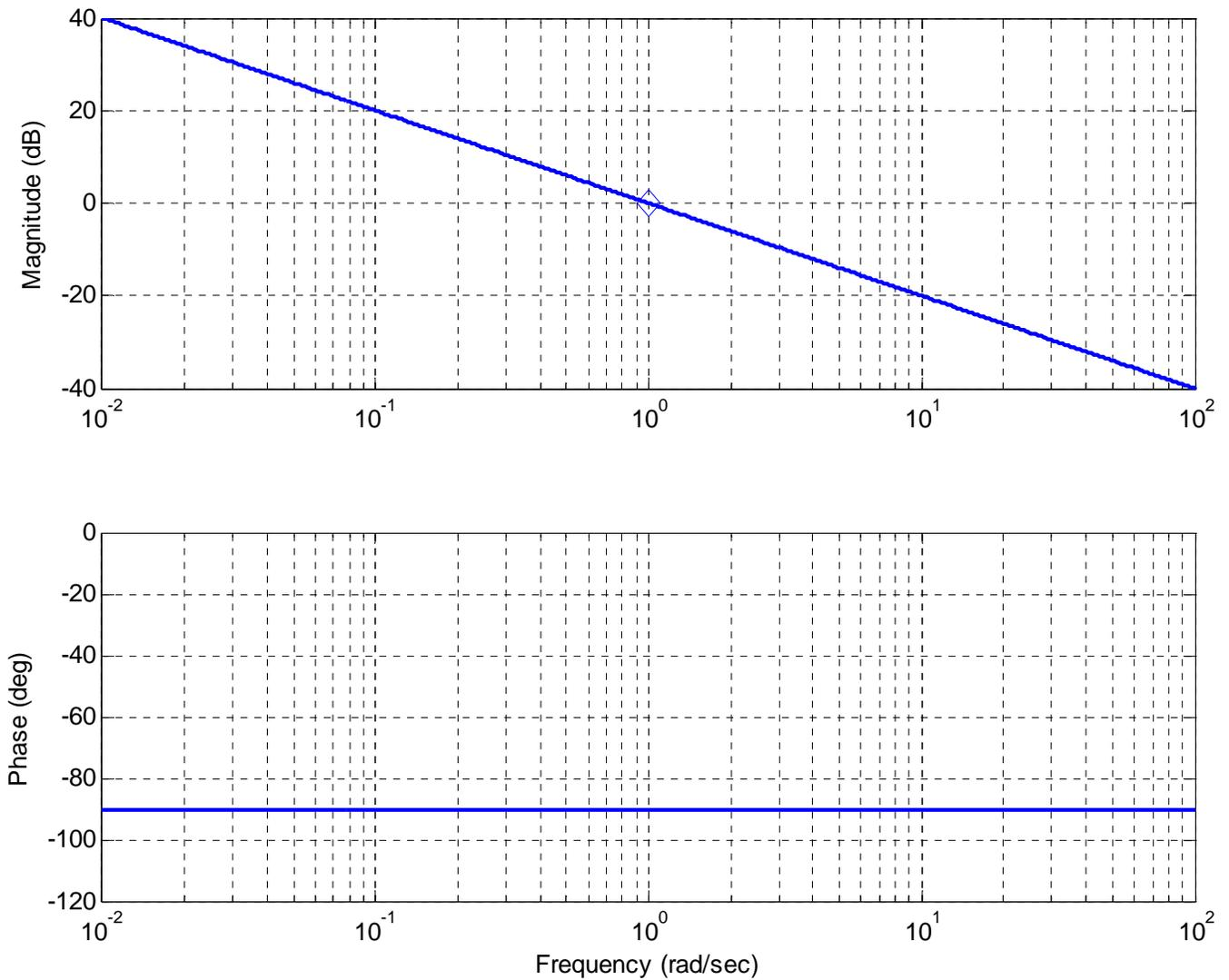
**Figure 8.10.** Bode plot of the transfer function  $G(s) = s^2$ . Note that that a diamond delineates the point (1 rad / sec, 0 dB).
