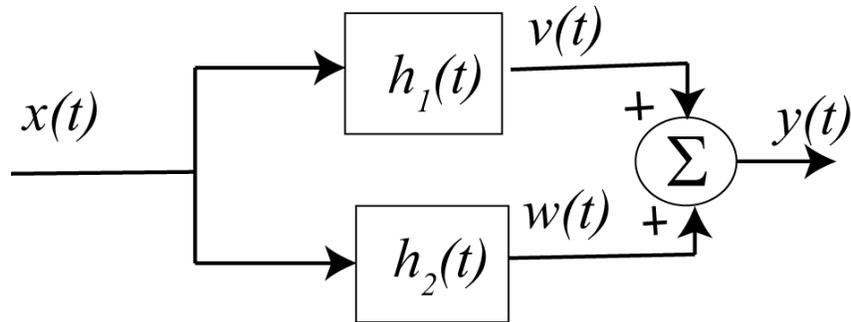
**Figure 5.22.** Two LTI systems connected in parallel.
