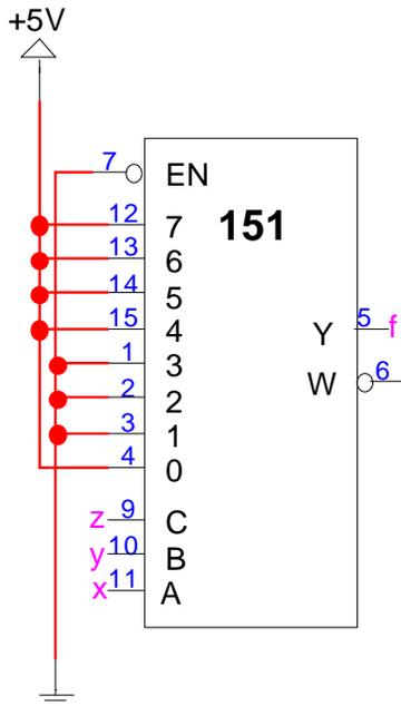
2. Implement a 32:1 multiplexer with active-low enable using only ONE 74LS151 multiplexer and any glue logic (AND, OR, NOT, etc.) that you desire. Build your circuit using simulation software. NOTE: you should not try to test this circuit with all  $2^{32}$  inputs!!!
