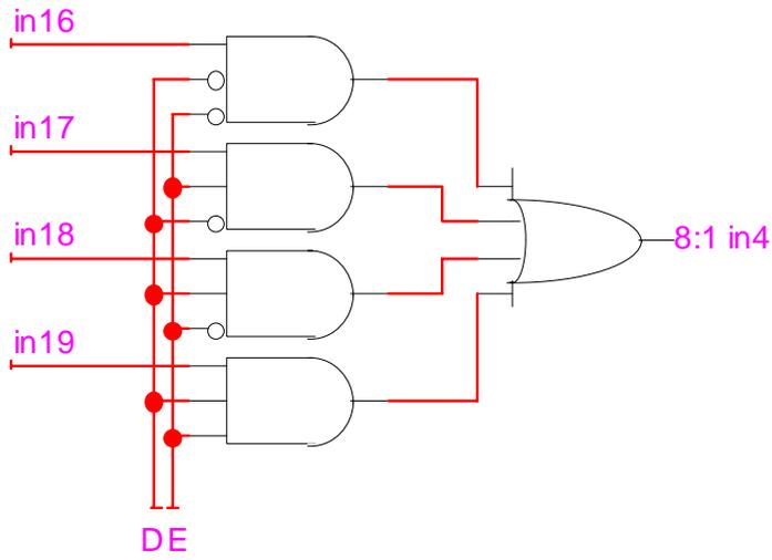
Making one sub-circuit for each of the eight inputs leads to the final circuit:
