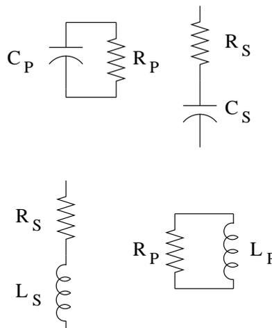
It's important to recognise that the values of the components in the two types of model are not equal, though they are related. For the capacitor,
