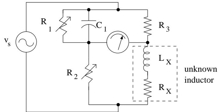
In Maxwell's bridge, resistors  $R_2$  and  $R_3$  remain as in Wheatstone's bridge, but a variable resistor  $R_1$  is placed in parallel with a standard (precisely known) capacitor  $C_1$ . A series model is used for the unknown inductor.
