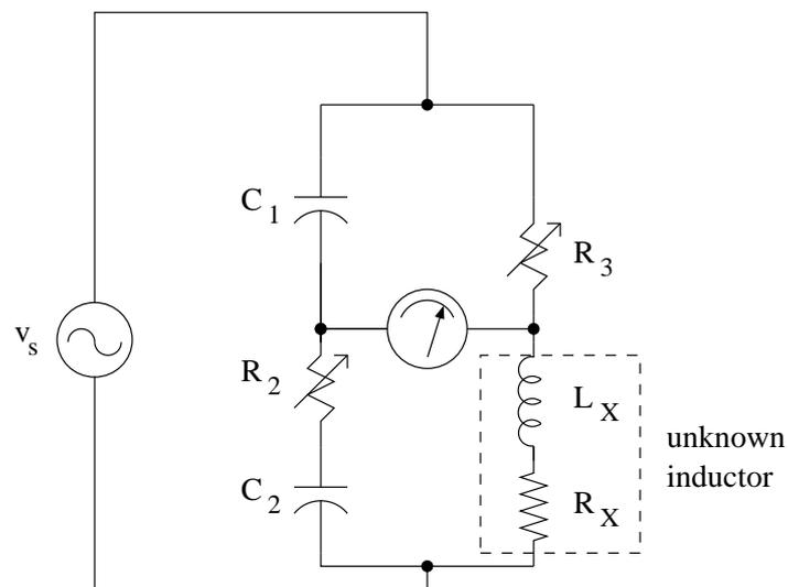
The balance equations for Owen's bridge are frequency independent:
