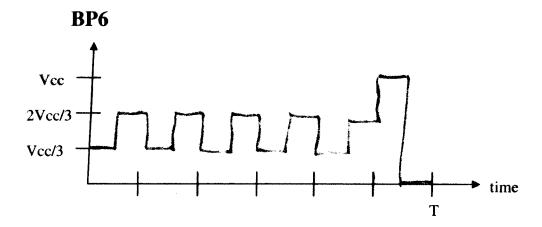
FPi (This waveform should turn ON Segments 1,3,5 and turn OFF Segments 2,4,6)
