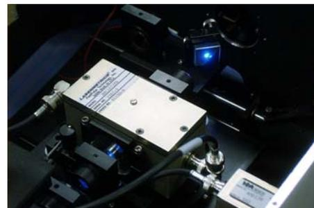
**k** Set the DC high-voltage bias to the Pockels cell for the highest modulation on S&R. This nearly always involves reducing the DC HV bias.
