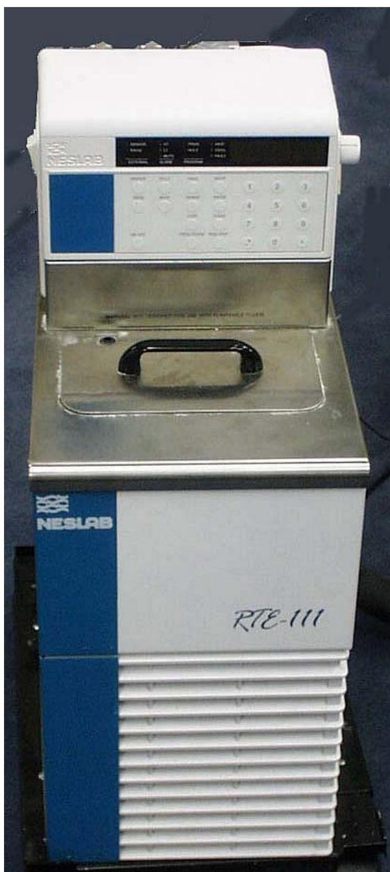
The F-1000/1 is offered as an accessory for maintaining sample temperature as well as for automating the measurement of temperature curves and other heating- or cooling-related assays. The bath is controlled by the host computer via a single serial (COM port) link. The bath may be used with water or a solution of ethylene glycol to control sample temperature from about  $-15$  to  $+80^{\circ}\text{C}$ . The F-1000 requires 110 V/60 Hz and the F-1001 uses 220 V/60 Hz line voltage.
