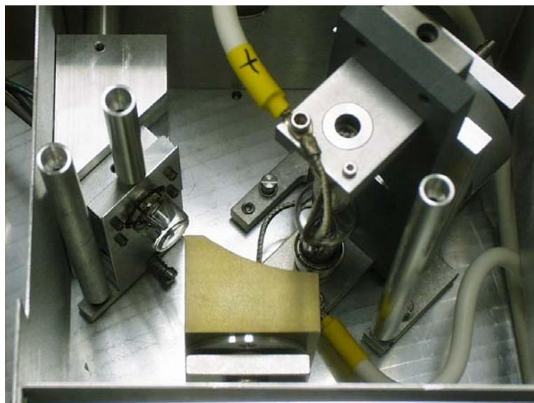
The phosphorimeter adds the ability to perform phosphorescence or delayed fluorescence measurements using a programmable pulsed-excitation source and selectable signal gating from the signal photomultiplier tube. This provides time-discrimination capability to remove competing luminescence emissions based on their lifetimes. The FL-1042 consists of a dedicated xenon flash-lamp housing, acquisition controller, and related electronics. The FL-1040 dual-lamp housing is required.
