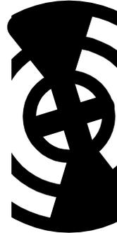
Rotation: poor polarizer alignment around Pockels cell
