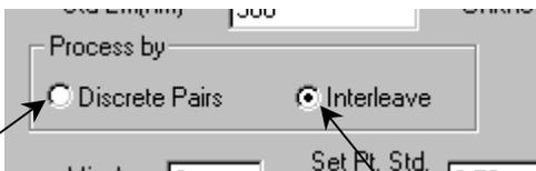
**Discrete Pairs** measures the phase-angle difference and demodulation of the standard, and then the unknown. From this, the computer saves the phase and modulation data and calculates lifetimes based on phase and modulation. Then, it repeats the procedure for the next average, measuring the standard, then the unknown, saving the data and calculating lifetimes. Thus, with discrete pairs, averages are non-shared measurements of the standard, followed by the unknown.
