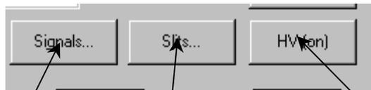
There are two possible signal choices that may be chosen in **Signals...** window: S & R or T & R (if available). The radio buttons show the detectors that may be selected for the lifetime scan. Choose the appropriate signal detector to be compared with the reference, **R**, detector for the lifetime acquisition.
