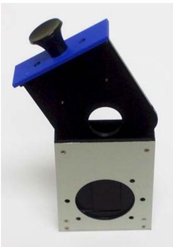
This emission filter-holder and spatial filter allows an emission lifetime detector to be mounted directly to the sample compartment without an emission monochromator in the light path. As the name implies, this accessory contains a filter-holder for 2" × 2" or 1" × 2" filters, and sets the emission detector at the appropriate focal length for the emission beam from the sample. The accessory also has a manual shutter to protect the detector from saturation.
