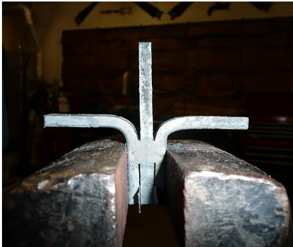
Figure 2: Blank after first set of bends, notice the spacers (left), finished snowflake (right)
