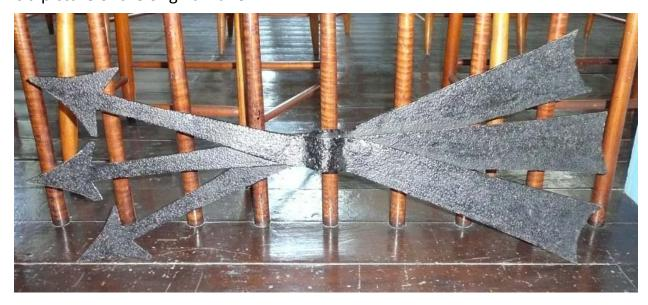
If you want to build your own, here are some construction notes. The vane consists of four parts. The back and front arrow are identical. Each is forged from a single piece of iron and looks like shown below. The top diagram gives a side view and the bottom diagram the top view.
