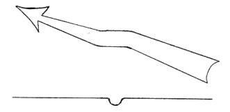
The middle arrow consists of two parts. Imagine a straight arrow cut in half. The three arrows are riveted together with four bolts, two on each side of the pivot. The rivet heads are flush with the arrows.
