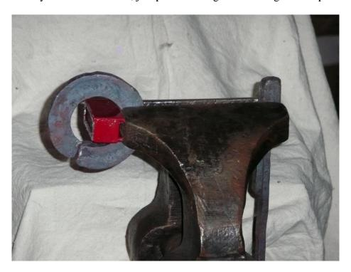
The wedge is made from a 5" piece of 3/4" mild steel, forged into an 8" long wedge. The wedge tapers gradually to about 1/16" thick. When bending the wedge into a circle, it helps to bend the thick side first. The magnet is about 2" long and can be purchased at Harbor Freight.
