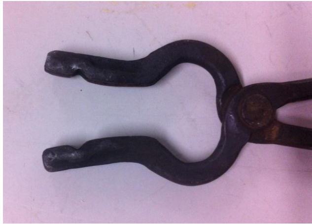
Figure 2: Off-Center brand V-bit tongs
