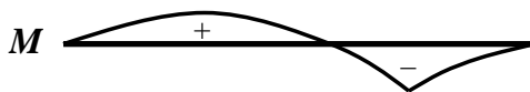
Figure 6. Example of how knowledge of deflected shape can be used to predict features of the moment diagram for a beam.
