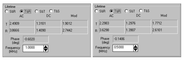
There is little difference between the two T-channel signals, the phase, and the modulation. Thus there is no advantage to including 0.5 MHz in the experiment, and the lower frequency limit is set to 1 MHz.
