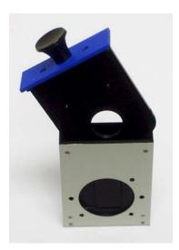
This emission filter-holder and spatial filter allows an emission lifetime detector to be mounted directly to the sample compartment without an emission monochromator in the light path. As the name implies, this accessory contains a filter-holder for  $2" \times 2"$  or  $1" \times 2"$  filters, and sets the emission detector at the appropriate focal length for the emission beam from the sample. The accessory also has a manual shutter to protect the detector from saturation.
