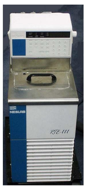
The F-1000/1 is offered as an accessory for maintaining sample temperature as well as for automating the measurement of temperature curves and other heating-or cooling-related assays. The bath is controlled by the host computer via a single serial (COM port) link. The bath may be used with water or a solution of ethylene glycol to control sample temperature from about –15 to +80°C. The F-1000 requires 110 V/60 Hz and the F-1001 uses 220 V/60 Hz line voltage.
