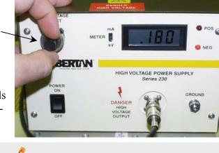
**Warning:** Do not increase the HV DC bias level to the Pockels cell above 350 V. Higher voltages can damage the Pockels-cell electronics.
