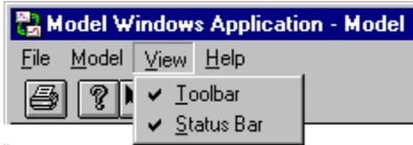
The *View* command displays or hides the toolbar and status bar. The status of each icon is listed in the drop-down menu: a check appears next to the toolbar or status bar if it is visible on the control panel.
