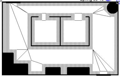
A <u>connectivity graph</u> is created using cell decomposition path planning. The space is divided into free and occupied cells. The trapezoidal decomposition of a space is shown below:
