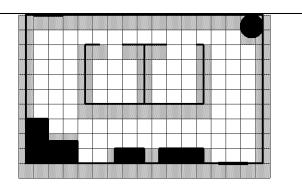
A \_\_\_\_\_\_ (adaptive cell decomposition) avoids wasted space because it is a recursive grid. It is one of the more popular techniques for mobile robot path planning. This is low computational complexity for path planning.
