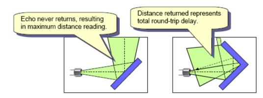
ECE497: Introduction to Mobile Robotics (C.A. Berry) -**Complex Sensors**   The results is that the distance measurement is too large and inaccurate
