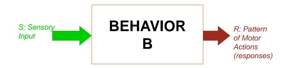
A behavior is a mapping of sensory inputs to a pattern of motor actions which are then used to achieve a task.
