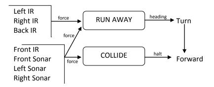
Figure 1: Level 0 – Obstacle Avoidance
