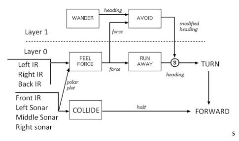
Figure 3: Subsumption Architecture - Obstacle Avoidance, Random Wander Example
