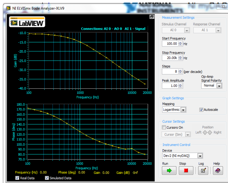
Figure 8: NI myDAQ design lowpass filter Bode Analyzer
