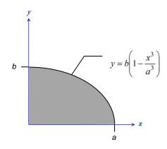
Find the *y*-centroid for the shape below. This time use a horizontal strip for the elemental area.
