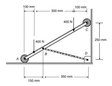
Draw FBDs of rope BD and link AC. (Hint: include the rollers.
