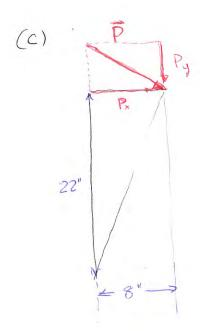
Moment is due to two pieces; the moment due to Px & the moment due to Px added with the correct signs.
