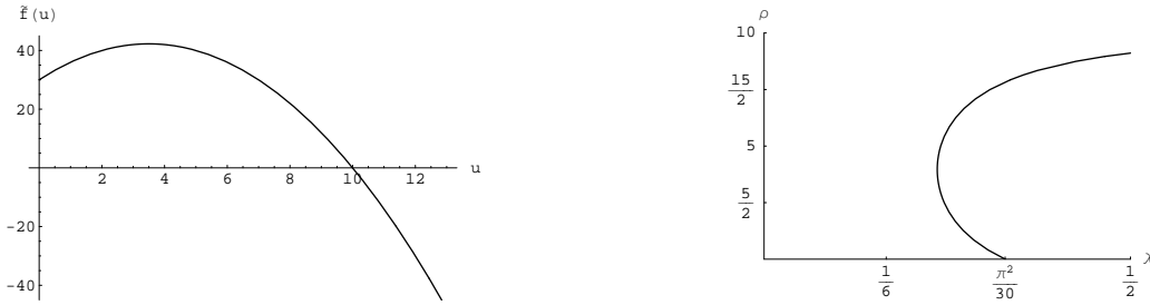
Figure 10: \tilde{f}(u) vs. u for \tilde{f}(u) = (u + 3)(10 - u) and the corresponding bifurcation diagram
