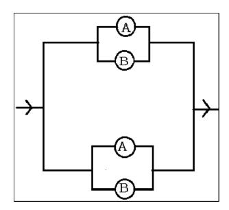
1.a Determine the system reliability function R(p,q) as a polynomial in p and q.
