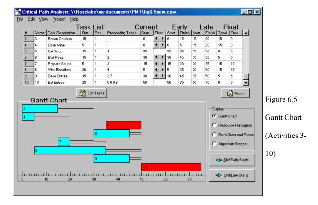
If you are still having difficulty understanding the differences between free and total float or are struggling with the Critical Path calculations, use the algorithm stepper in the CritPath program. It will walk you through the process using a graphical representation (see Figure 6.6).
