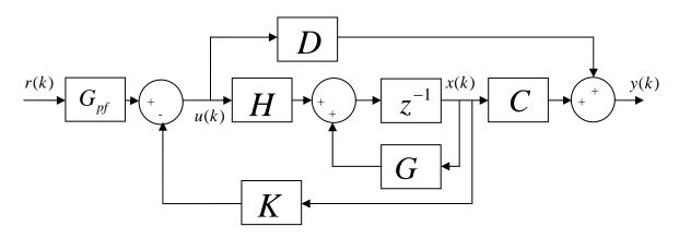
Here  $G_{pf}$  is the <u>prefilter gain</u>, r(k) is the <u>reference input</u>, and  $K = \begin{bmatrix} k_1 & k_2 \end{bmatrix}$  is the <u>feedback gain matrix</u>. The state variable model for the plant is assumed to be
