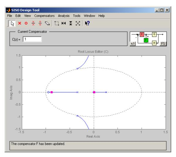
Next we have to try an I controller for C(z). Let's assume  $C(z) = \frac{K_i}{1-z^{-1}} = \frac{K_i z}{z-1} = \frac{0.1 z}{z-1}$ .
