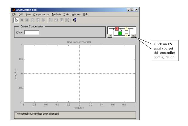
Sisotool will allow us to modify both C(z) and F(z), but it is much easier to modify C(z). We will have to iterate between both of these.
