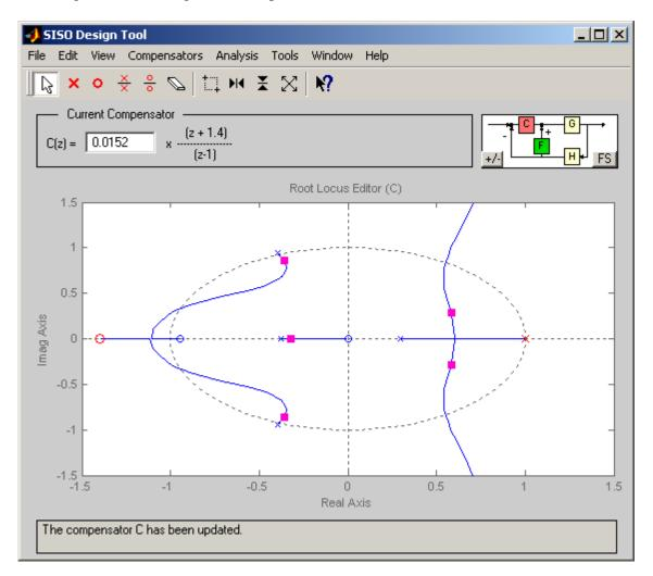
At this point we can drag the zero around and also drag the red squares around (which change the gain value). However, we can do nothing to change F(z) except to edit it. The step response for this controller configuration is shown on the following page:
