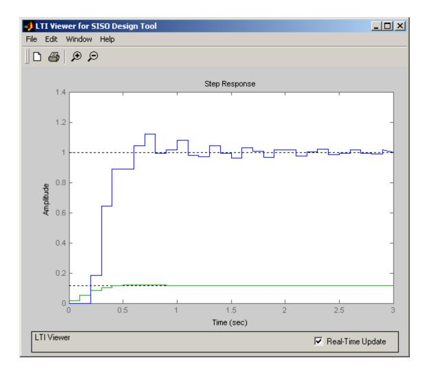
Note that, compared to a normal PID controller, the control effort is not infinite at 0, and actually builds as time goes on (like an integral controller). At this point we might want to go back modify C(z) to see if we get acceptable performance. If we cannot get acceptable performance we may then have to try another value for F(z).
