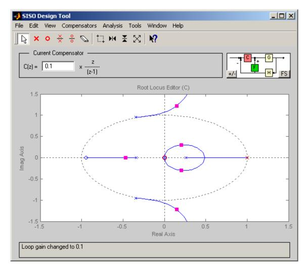
This is clearly an unstable system, so we need to change something! With the C(z) we can only change the gain, which will not help us here (we have two poles outside the unit circle with no way to get in). Clearly we must change F(z). After some playing around, I ended up with
