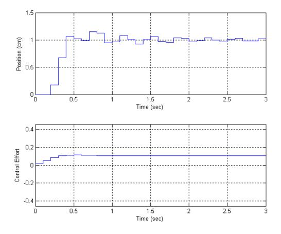
*I-PD Controller:* Now we'll assume we want to control the same plant, but this time use an I-PD controller. We first have to guess a PD controller. As a start, we'll try the following PD controller
