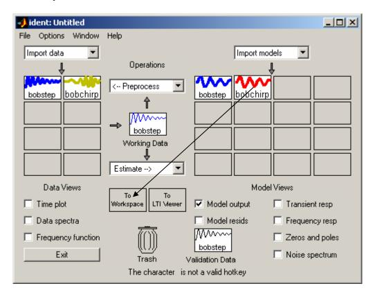
Now our workspace has access to the discrete-time model. Next we need to load the data we want to test our model against. This is important since it gives us the system input and time vector. If we are going to test against a step input, type
