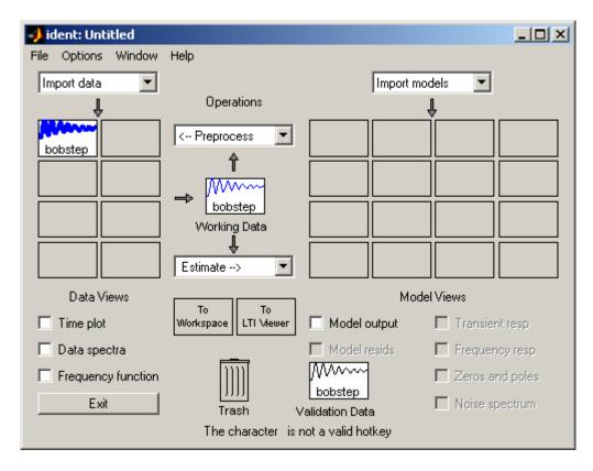
At this point we are ready to use the data to make our first discrete-time model. Since the only data that we have is from **bobstep**, that becomes the *Working Data*. To change the *Working Data*, we just drag a data set over to *Working Data*, as you will see.
