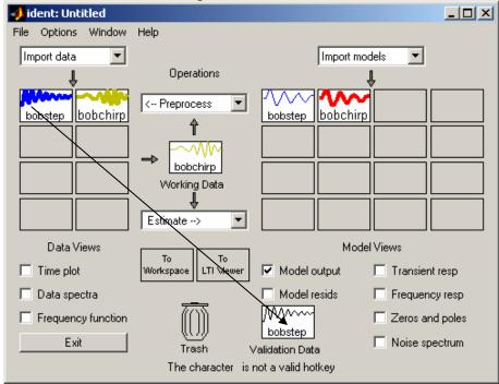
At this point, we can see how our newest model, **bobchirp**, matches the measured output when the input is a step. As these figures show, there is an offset between the model output and the measured output for this input. This is fairly common for these systems, and there are some ways we can try to fix this, which we will mention later in this lab.
