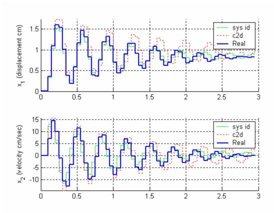
Here we see the response of the model created using the system identification toolbox( sys id), the response of the model made discretizing your continuous time model (c2d), and the response of the real system (Real). The color schemes looked good to me, but feel fee to modify them. If you do change color schemes or line types, be sure they print well in black and white (unless you print your memos in color!)
