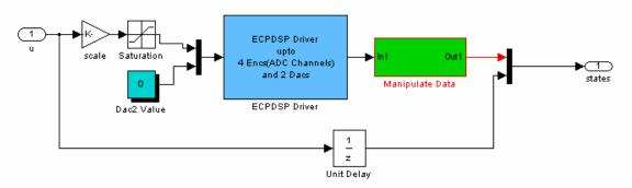
The top two state coming out of the system will be `real states', while the bottom state will be a delayed version of the input u(k-1). If we look inside the *Manipulate Data* block, we see the following:
