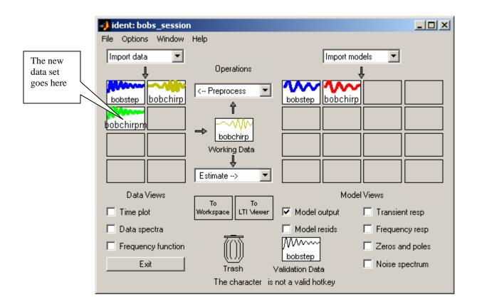
You can now use the merged data set to construct a new model, and the response of the new model to any of the other data sets. Note, however, that sometimes merging files does not produce a better model than the two individual files did.
