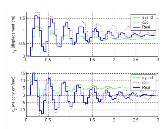
Here we see the response of the model created using the system identification toolbox(sys id), the response of the model made discretizing your continuous time model (c2d), and the response of the real system (Real).
