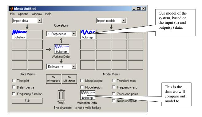
We should now look at how closely the model matches our input. To do this, be sure **Validation Data** has the same name as the input data set. The click on **Model output.** The following is what I got (for a 3 second sample):
