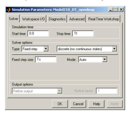
Ts and Tf are set by **DT\_openloop\_driver.m**, though you may want to change the final time in Matlab's workspace. I would suggest a final time (Tf) of between 3 and 20 seconds or so, it really depends on your input to the system.
