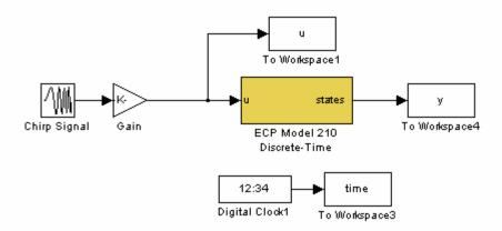
The parameters I used for my system is shown below, with a gain of 0.01. You should note that we are using very low frequencies since our system cannot really respond very quickly.
