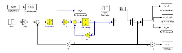
For the pulse generator *disturbance*, set the Amplitude to 0.2 cm, the Period to 2 seconds, the Pulse Width to 10%, and the Phase Delay to 1 second.
