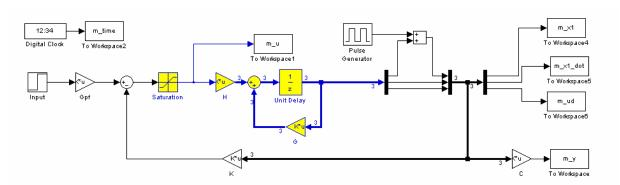
For the pulse generator *disturbance*, set the Amplitude to 0.2 cm, the Period to 2 seconds, the Pulse Width to 10%, and the Phase Delay to 1 second.
